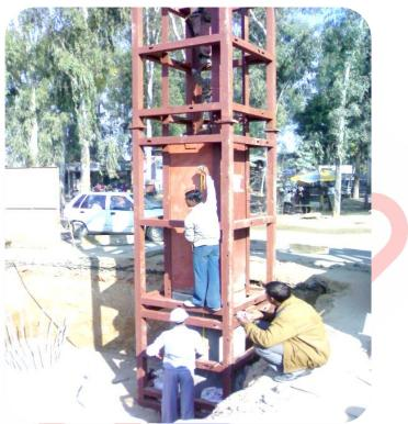
from 1m to 3m. A 25mm thick plywood cushion and 16mm thick steel plate were placed on the pile top to avoid any damage to the pile during testing. The testing procedure as per ASTM D4945
